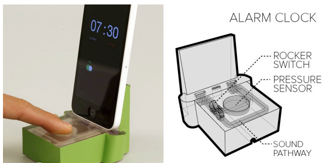
Figure 16. Our alarm clock application utilizes several mechanisms for interactive control, including a rocker switch and a pressure sensor.
