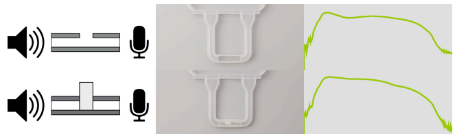
Figure 5. Open (top) and blocked tubes.
