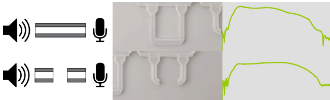
Figure 8. Physical gaps along the speaker-microphone pathway allow the audio signal to disperse into open air.
