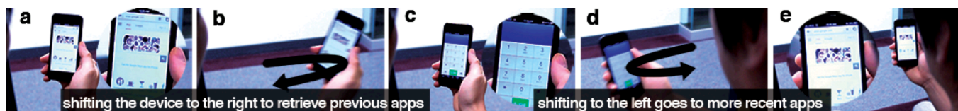
Fig 5. Around-body interaction enables multitasking between previous and more recent apps.
