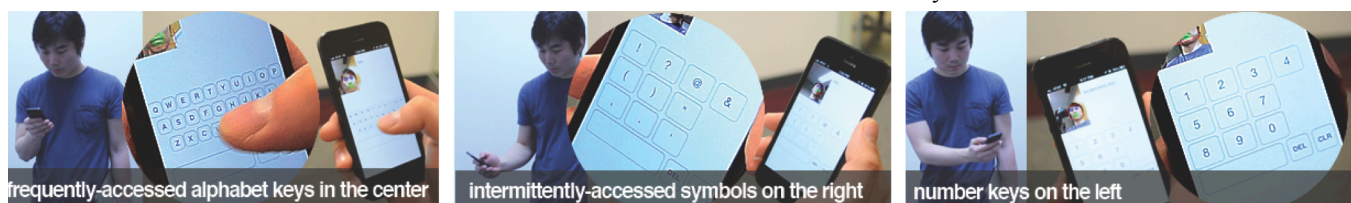
Fig 3. Around-body interaction maps a physical keyboard around the body
