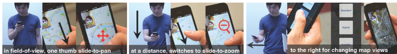
Fig 6. Around-body interaction mediates mode switching in a map app.
