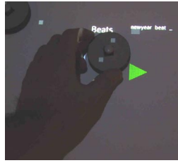
Figure 9a. The user presses the button on a puck to change its effect settings.
