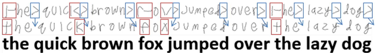
Figure 4. A sequence of strokes (top) can be formed into characters, words, and ultimately sentences (bottom). A ‘>’ character acts like a space bar (blue highlight). Strokes from multistroke characters (t, k, f, x) are spatially merged (red highlight).
