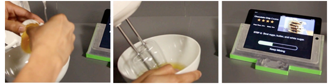
Figure 16. Object sensing enables rich, context-sensitive applications. For example, we can sense equipment used in the preparation of a meal (left). A progress bar informs the user when to stop blending ingredients.
