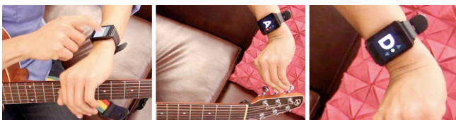
Figure 17. For an unpowered object e.g. , an acoustic guitar, we can detect the closest note to tune the instrument precisely.
