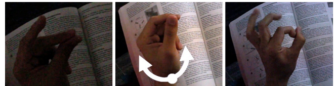
Figure 14. A snap turns on the nearest light. A pinch gesture followed by rotation of the wrist offers continuous brightness control. A flick confirms the manipulation.
