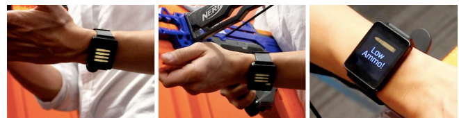
Figure 18. We can augment “analog” experiences with “digital” interactivity. With a Nerf gun, we can detect users loading ammo clips (left) and firing darts (middle).
