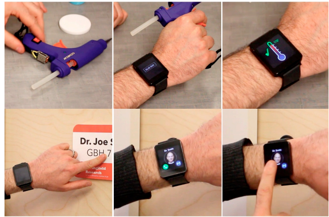
Figure 19. Vibro-tags emit structured vibrations that carry data. For example, the user can touch an office nameplate instrumented with a vibro tag (top), which transmits the person’s contact details to the smartwatch. We can also instrument non-mechanical objects, e.g., a glue gun (bottom). The tag broadcasts an object’s ID and metadata — in this case, the current temperature and ideal operating range.
