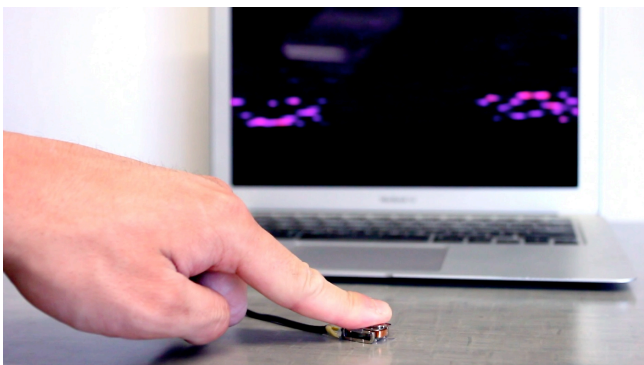
Figure 7. A “vibro-tag” transmitting FSK bio-acoustic data through the user’s arm, and received by the smartwatch.
