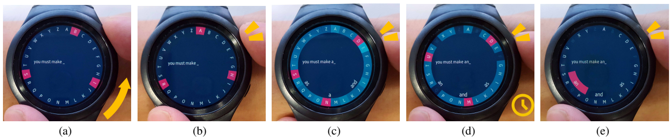
Figure 1: A storyboard illustrating a user entering “an” with COMPASS . (a) The keyboard shows three cursors at initial locations, the user rotates the bezel counterclockwise to hit ‘a’ with a nearby cursor. (b) The user presses the physical button to select ‘a’. (c) Upon selection, the keyboard changes the location of the cursors so as to minimize the expected rotational distance for the next key. As there is already a cursor on ‘n’, the user presses again to select ‘n’ without rotating. The color of each key indicates the probability of it being the next selection. (d) The user long-presses the physical button to enter word selection mode. Dimmed keys are not possible for the next selection. (e) The user presses the button to select “an”.
