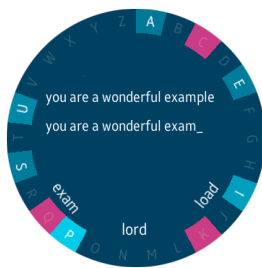
Figure 3: Visual cues to help users find the target keys. Impossible keys are dimmed, while others are highlighted according to their possibility.
