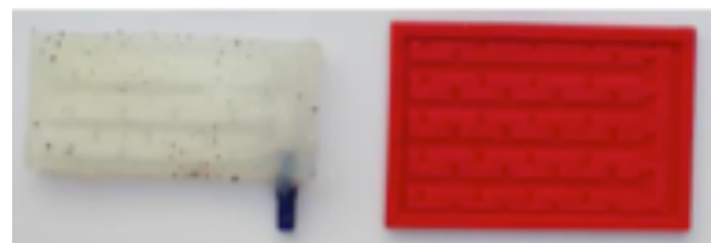
Figure 12. (Left) Patch with channels (filled with flour for better visual). (Right) 3D printer mold used to generate the bladder with silicon.
