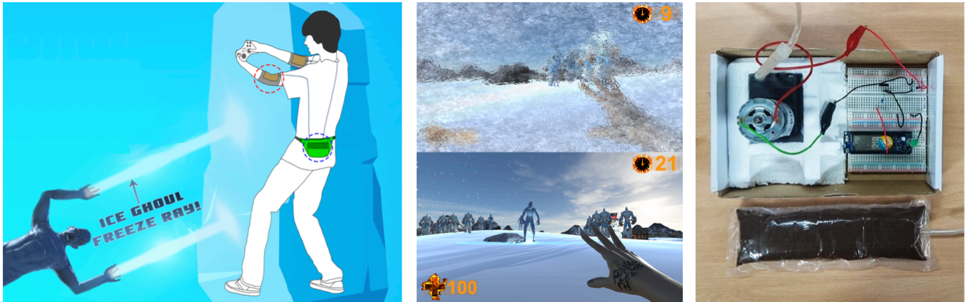
Figure 1. (Left) Frozen Suit can provide physical feedback in games by restricting users' movements, (Middle) for example giving the sensation of being frozen by an enemy. (Right) A jamming patch of the suit placed at a joint to restrict it.
