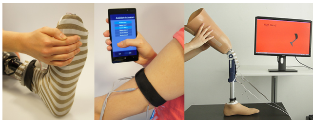
Figure 11. Customization allows for mapping custom regions dynamically to actuators via a mobile app (left, middle). The knee guard detects the degree of bending of a knee-joint (right).
