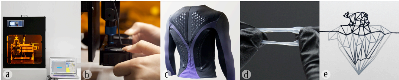
Figure 1: xPrint system. (a) Open hardware and software platform; (b) Magnet assembly based modular design and alignment; (c) Outcome of one user test: a sweat activated transformable garment; (d) Printed pH responsive calcium alginate gel sample; (e) Outcome of one user test: an animated painting on paper.
