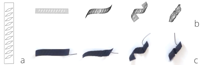
Figure 10. Given an encoded composite (a), our simulator is used to predict the inflated shape of the structure (b), which is in close agreement with the actual physical performance of the fabricated artifact (c).
