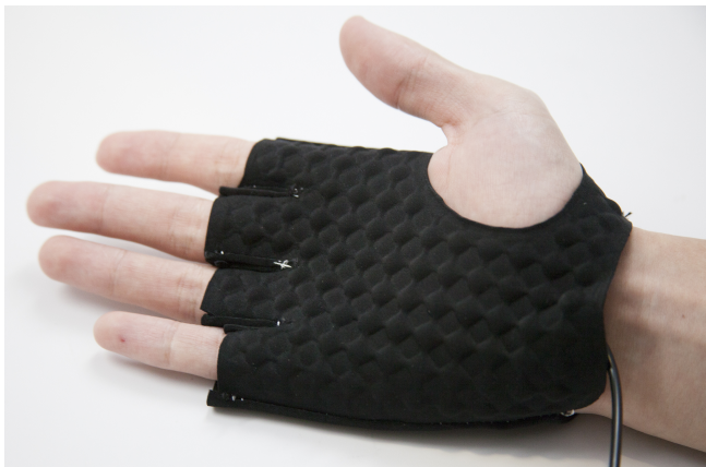
Figure 34. Biking gloves with changing surface texture on the palm. Gloves are made with cotton fabric.
