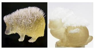
Figure 12. Printed figures with controllable hair stiffness.
