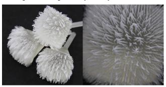
Figure 9. Successful printed hair arrays on curved surfaces.
