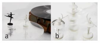
Figure 26. (a) Printed dancing figures on our customized speaker/dancing table. (b) Ballet dancers rotate in different velocity due to the difference in the tilting angle of the hair structure.
