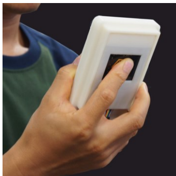
Figure 1. Appearance of the device with a user. The electro-tactile display on the back of the smartphone presents a shape-touching sensation to the index finger of user.
