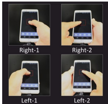
Figure 5. Experimental conditions. "Right" or "Left" represents a right or left hand holding the device. "1" or "2" represents, the case where only one hand is used for holding and operating the device or both of two hands are used, one is for holding and the other is for operating the device. For one hand case, the thumb of device holding hand is used as an operating finger.
